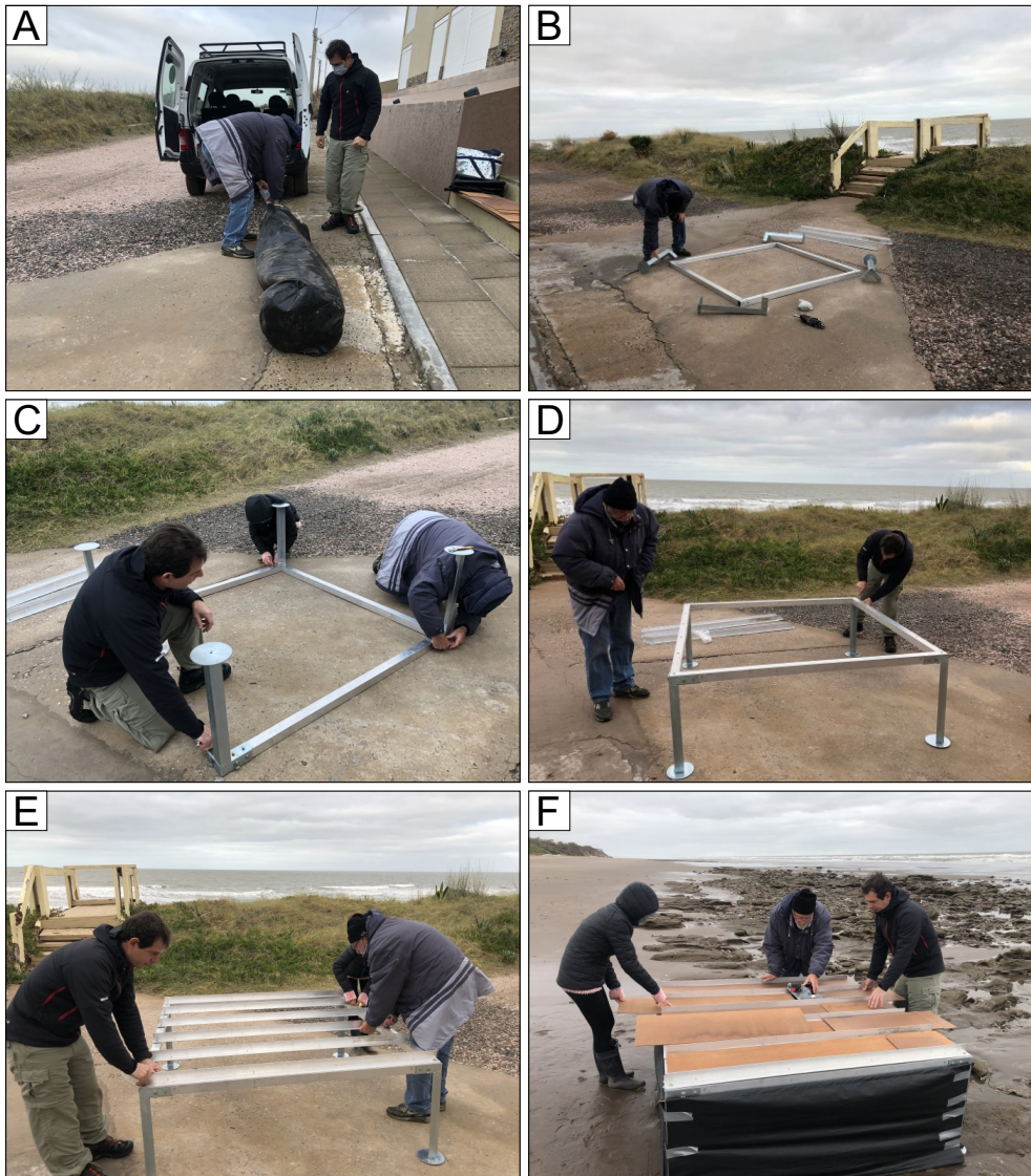
Figure 2. MiSMoS assembly stages. a) Storage of MiSMoS pieces, b) pre-assembly inspection of the structure, c) addition of supports and screws, and d) placement of supports for curtains. e) Incorporation and adjustment of aluminum rails to the MiSMoS structure frame, and f) movement of the sensor-carrying and panels that block light during the survey.
